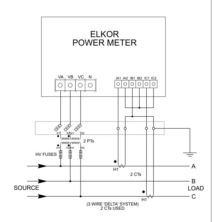
INTERFACING BLOCK (OPTIONAL) INCLUDING "DEAD-FRONT" FUSE BLOCK AND CT SHORTING MEANS (SEE DRAWING CODE: I-BLOCK)
